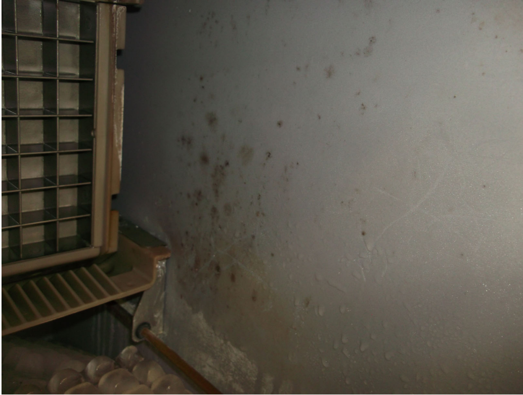
PHOTO 11 – 11/29/2022 PHOTO SHOWING VISIBLE MOLD GROWTH ON TH METAL WALLS OF THE ICE MACHINE.
