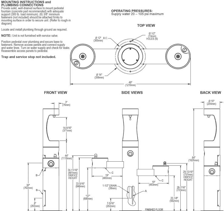
A = 3/8" O.D. Unplated copper tube connect. Shut off valve by others.
