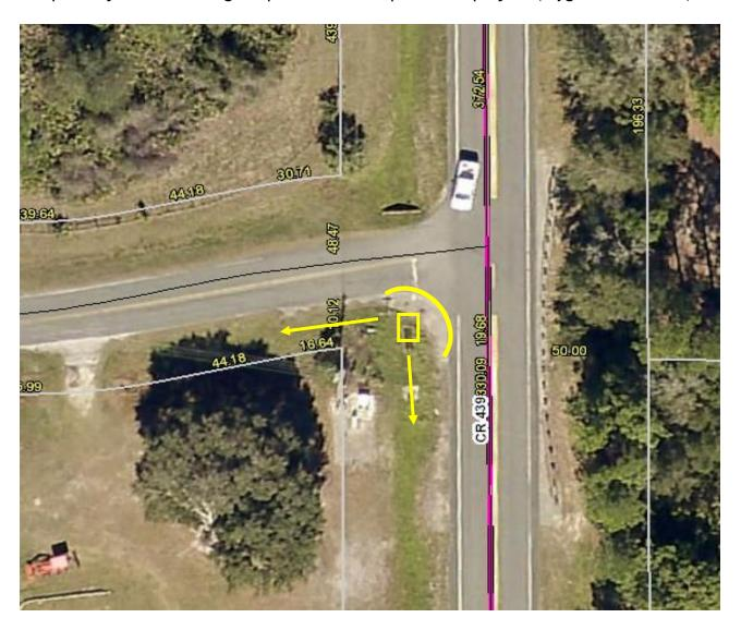
The contracted vendor shall remove and replace the existing 24" x 38" ERCP concrete pipe and install a pre-fabricated Type J drainage structure. The existing swale shall be regraded for positive drainage.
