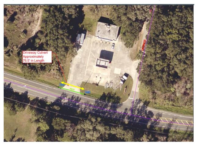
The contracted vendor shall remove the existing driveway and 18" CM pipe and replace with 18" HDPE pipe with concrete mitered ends. The concrete driveway shall be constructed with 6 inches of reinforced concrete (4000 PSI) using 10 foot square of 6 inch by 6 inch wire mesh extending a minimum of 10 feet from edge of existing pavement. Swales shall be regraded to allow for positive roadway drainage and sod with Bahia.
