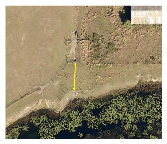
This project shall consist of re-grading the existing drainage easement and placement of 24" x 38" ERCP pipe with concrete mitered ends. The project shall include placement of concrete rubble and the installation of geotextile turf reinforcement. This project includes the removal and replacement of four foot barb wire fencing and installation of five foot galvanized chain link fencing with access gates. All disturbed areas shall be sodded using Bahia sod.
