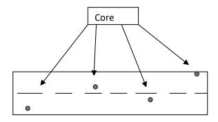
2.41. The results of the core sample tests shall be sent directly from the laboratory to the County's Project Manager. From these samples, a determination of the average thickness of the asphaltic concrete shall be made by the testing laboratory. If at any time Contractor wishes to request more core samples than what the County has required, they shall do so in writing. The cost for the additional cores shall be the responsibility of Contractor.
