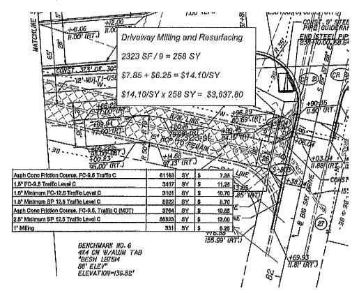
I get value of milling and resurfacing at \$3,637.80 per original plan. Area at 258 SY. Was 390 SY value measured length of full driveway.
