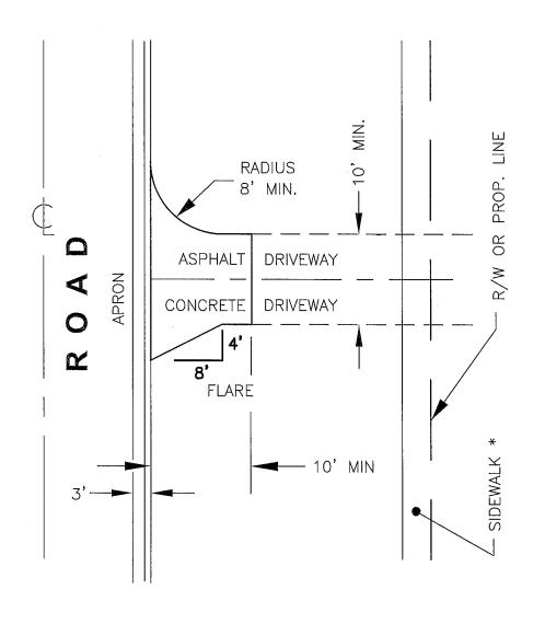
\* SIDEWALK (IF REQUIRED) SHALL BE CONSTRUCTED TO MEET FDOT INDEX 310, ADA SPECIFICATIONS SPECIFICATIONS FOR PUBLIC RICHT-OF-WAYS, AND LAKE COUNTY STANDARDS WITH A MAXIMUM CROSS SLOPE OF 1.5% AND A MAXIMUM RUNNING GRADE SLOPE OF 5%, OFFSET 1' FROM PROPERTY LINE/ RICHT-OF-WAY LINE.
