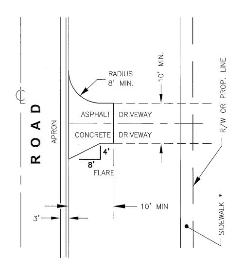
SIDEWALK (IF REQUIRED) SHALL BE CONSTRUCTED TO MEET FDOT INDEX 310, ADA SPECIFICATIONS SPECIFICATIONS FOR PUBLIC RIGHT-OF-WAYS, AND LAKE COUNTY STANDARDS WITH A MAXIMUM CROSS SLOPE OF 1.5% AND A MAXIMUM RUNNING GRADE SLOPE OF 5%, OFFSET 1' FROM PROPERTY LINE/ RIGHT-OF-WAY LINE.
