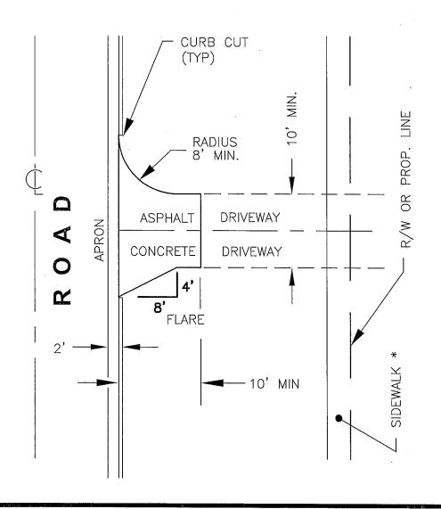
SIDEWALK (IF REQUIRED) SHALL BE CONSTRUCTED TO MEET FOOT INDEX 310, ADA SPECIFICATIONS SPECIFICATIONS FOR PUBLIC RIGHT-OF-WAYS, AND LAKE COUNTY STANDARDS WITH A MAXIMUM CROSS SLOPE OF 1.5% AND A MAXIMUM RUNNING GRADE SLOPE OF 5%, OFFSET 1' FROM PROPERTY LINE/ RIGHT-OF-WAY LINE.
