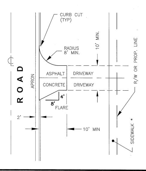
SIDEWALK (IF REQUIRED) SHALL BE CONSTRUCTED TO MEET FDOT INDEX 310, ADA SPECIFICATIONS
