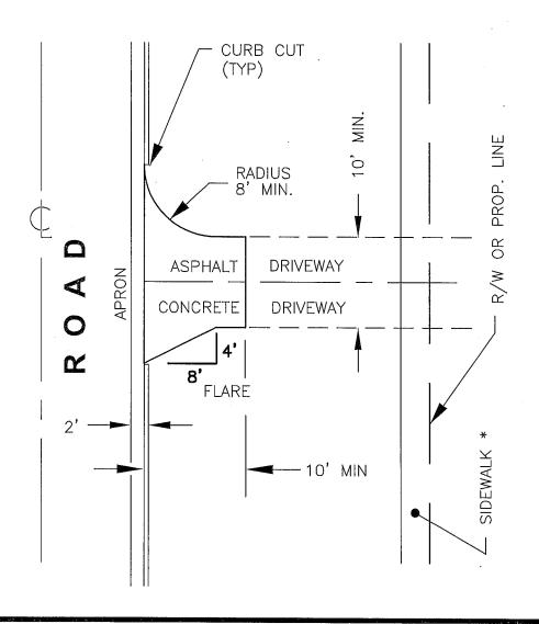
SIDEWALK (IF REQUIRED) SHALL BE CONSTRUCTED TO MEET FDOT INDEX 310, ADA SPECIFICATIONS SPECIFICATIONS FOR PUBLIC RIGHT—OF—WAYS, AND LAKE COUNTY STANDARDS WITH A MAXIMUM CROSS SLOPE OF 1.5% AND A MAXIMUM RUNNING GRADE SLOPE OF 5%, OFFSET 1' FROM PROPERTY LINE/ RIGHT—OF—WAY LINE.
