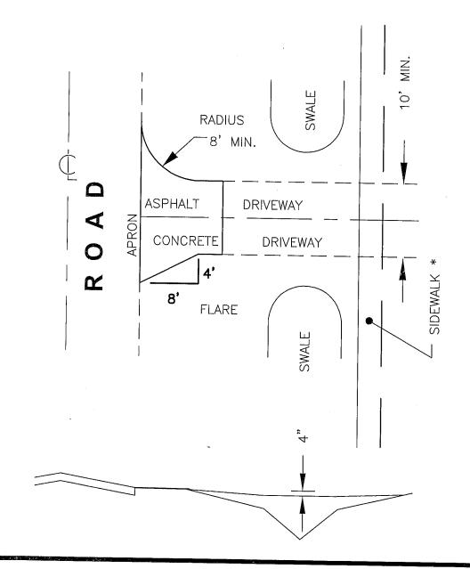
SIDEWALK (IF REQUIRED) SHALL BE CONSTRUCTED TO MEET FDOT INDEX 310, ADA SPECIFICATIONS SPECIFICATIONS FOR PUBLIC RIGHT-OF-WAYS, AND LAKE COUNTY STANDARDS WITH A MAXIMUM CROSS SLOPE OF 1.5% AND A MAXIMUM RUNNING GRADE SLOPE OF 5%, OFFSET 1' FROM PROPERTY LINE/ RIGHT-OF-WAY LINE.
