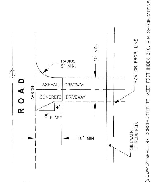
1. 1" ASPHALT W/6" COMPACTED LIMEROCK BASE.
