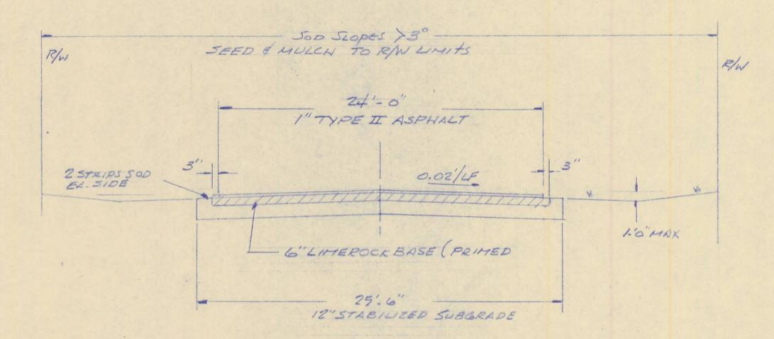
ROAD SECTION - NEW CONSTRUCTION STAT 22+17 TO STAT 26+07
