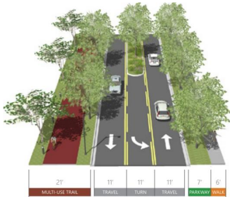
Figure 13 - Proposed Complete Streets in Wolf Branch Innovation District |Source: Wolf Branch Innovation District Master Plan
