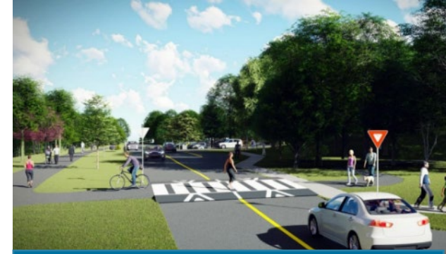
Raised Side Street Crossing
