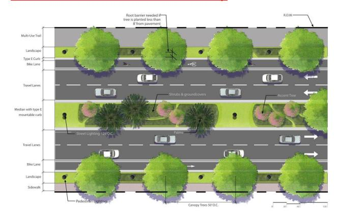
c. <u>Urban Section – Optional Trail Configuration in WWAP Center with</u> Buildings at Edge of Right of Way.
