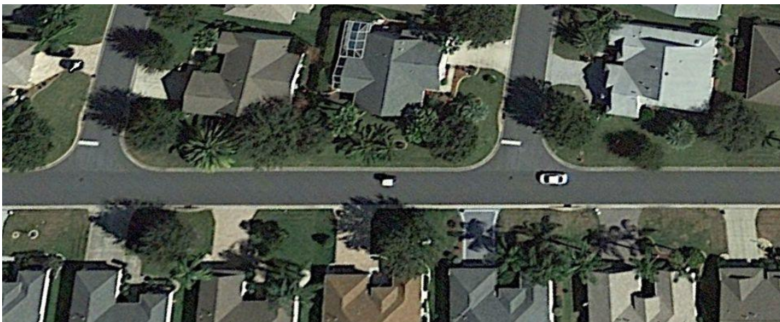
Figure 11: Local Roads – typical residential neighborhood roads with very low traffic volume, frequent intersections and driveways
