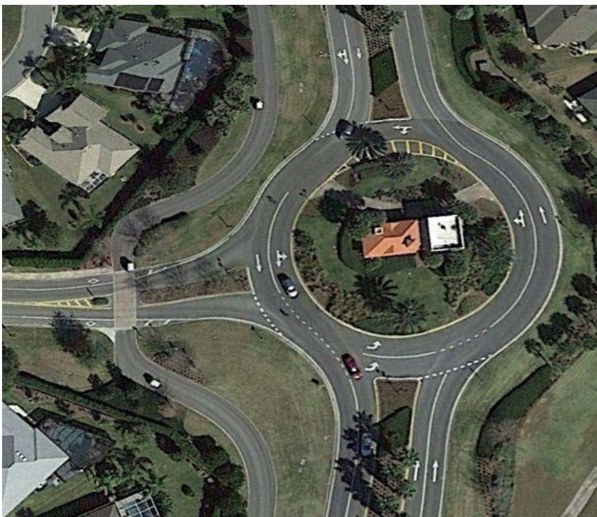
Figure 21: Typical 3-way traffic circle
