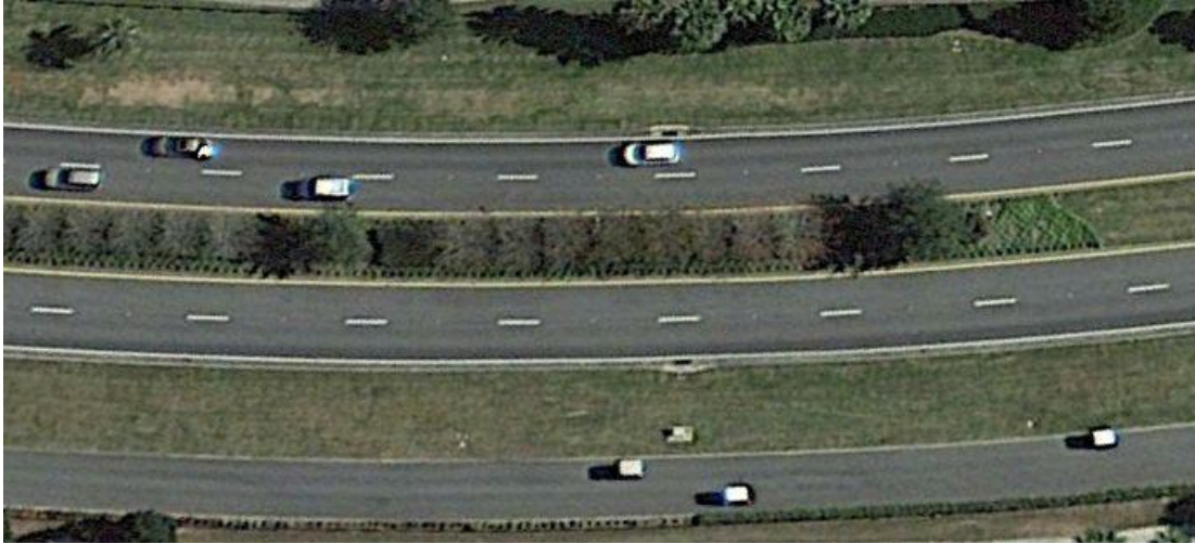
Figure 6: Arterial Road example: Morse Boulevard (35 mph), with 4 vehicle lanes, center island and parallel multi-modal path
