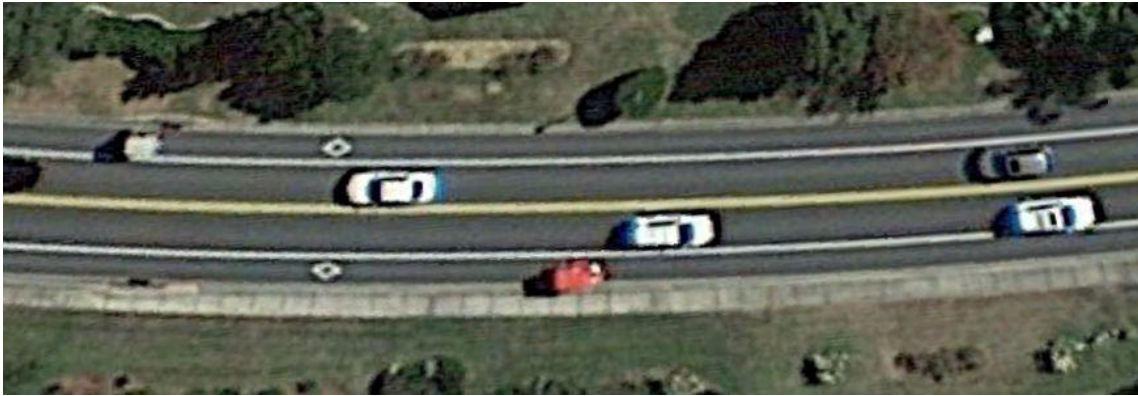
Figure 9: Typical Collector Road, with two regular vehicle lanes and two cart/bike lanes
