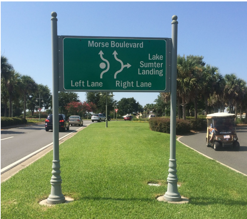
Figure 29: Typical traffic circle instruction sign
