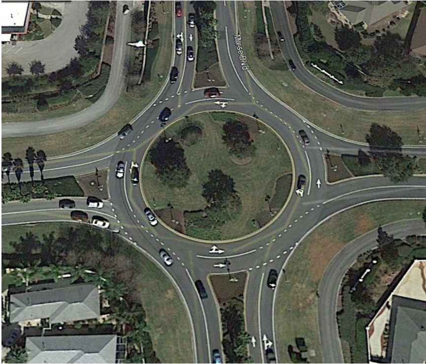
Figure 20: Typical 4-way traffic circle
