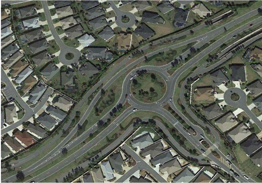
Figure 22: Typical traffic circle: 3-way with bypass lane
