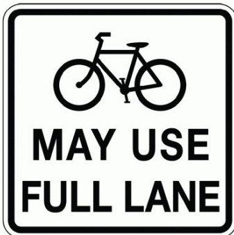
Figure 37: May Use Full Lane sign
