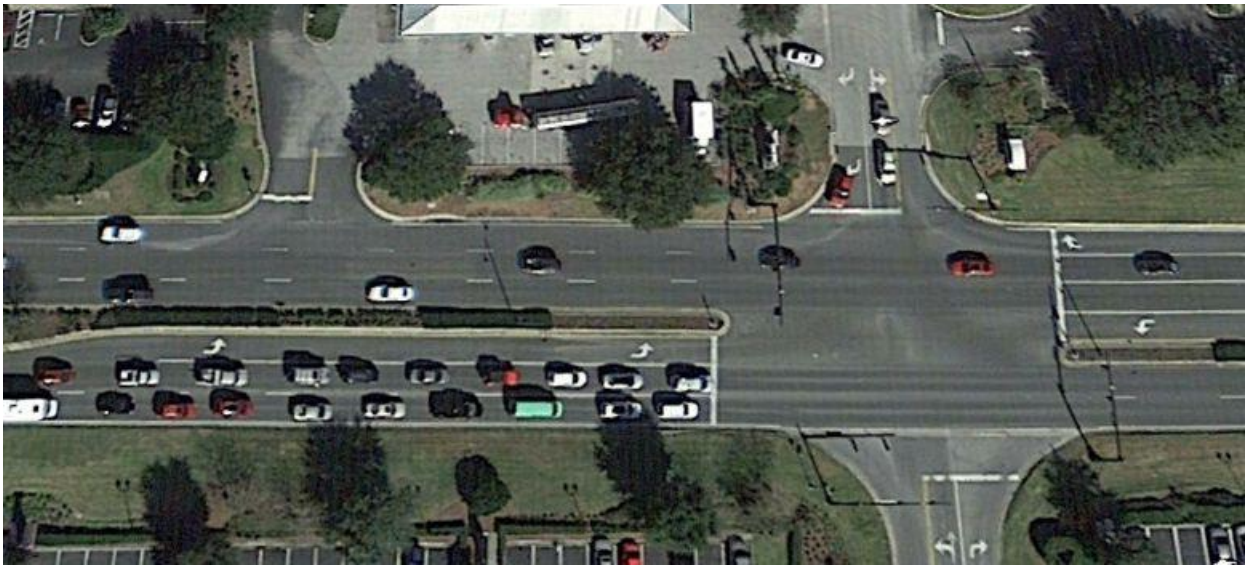
Figure 8: CR466 west of Buena Vista Boulevard, with congestion from turn lanes, multiple entrances and intersections, not suitable for bicycles
