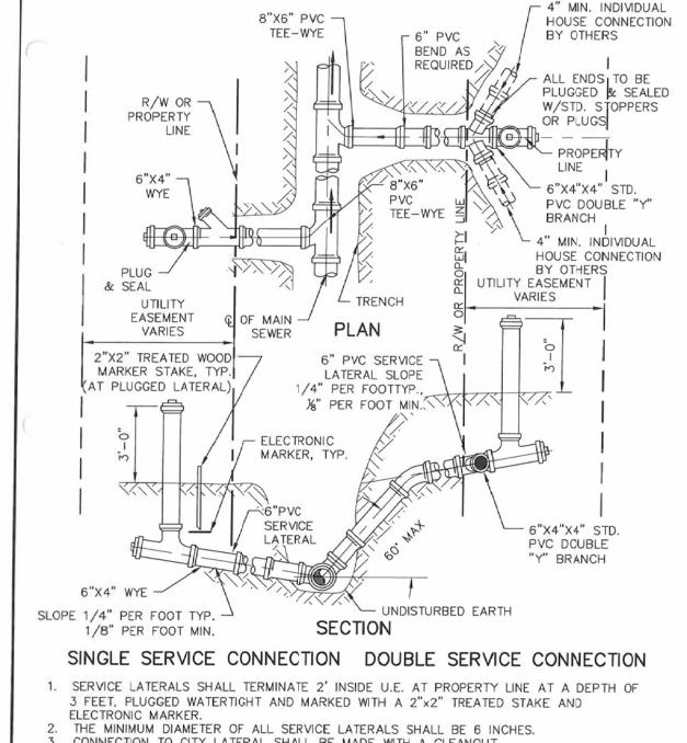
CONNECTION TO CITY LATERAL SHALL BE MADE WITH A CLEANOUT.
