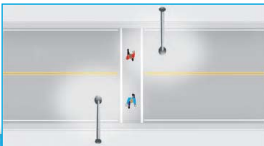
Proper placement of crosswalk illumination (Credit: Michele Weisbart, Model Design Manual for Living Streets , Los Angeles County, 2011 )
